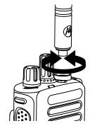
2 To remove the antenna, turn the antenna counterclockwise.
